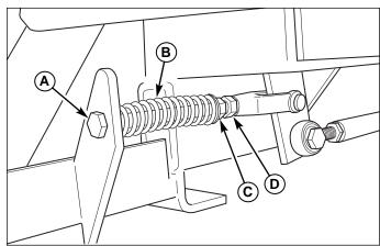
Figure 32. Neutral Spring Return Adjustment
